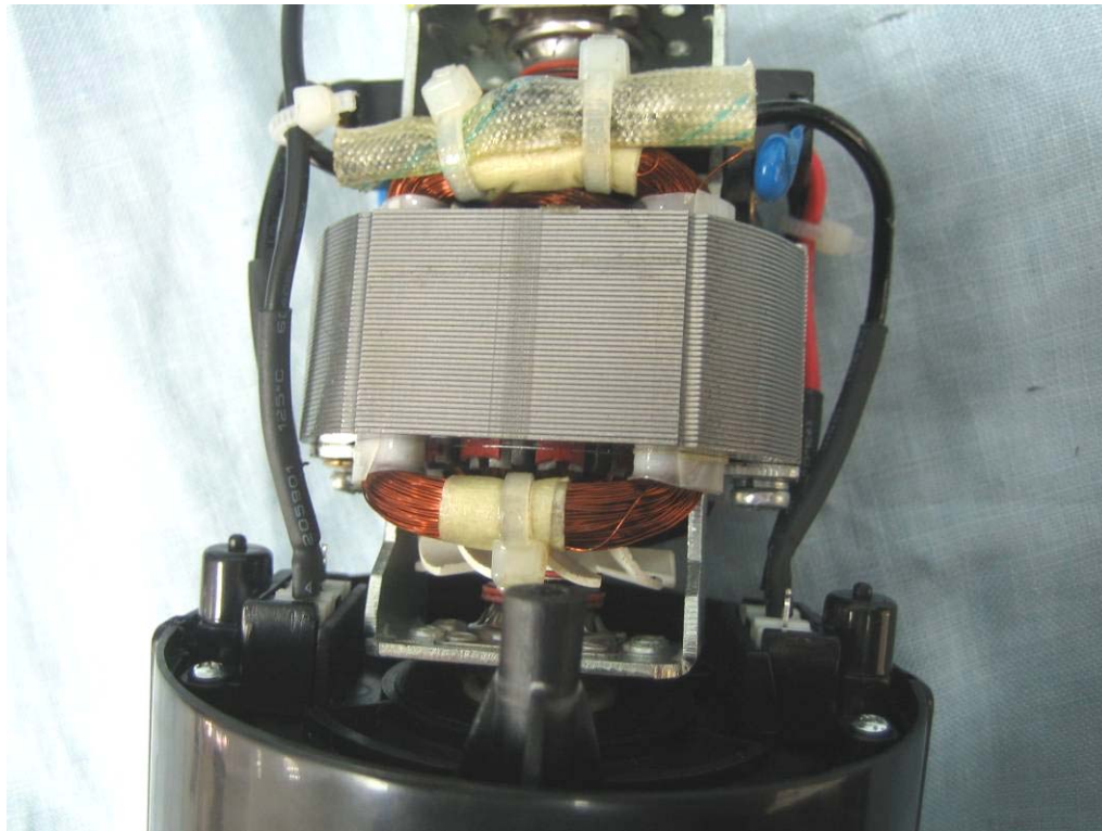
Earthing connection on the motor of coffee mill
