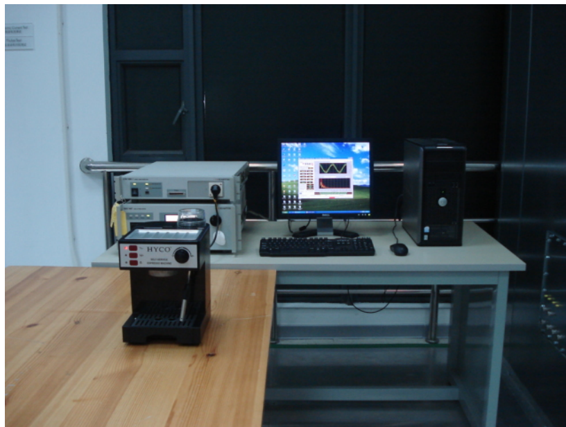
Figure 13 Setup for Harmonic current emission and Voltage fluctuations and flicker
